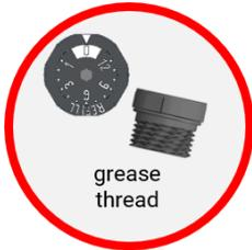
Take a new cartridge and grease the thread, e. g. with silicone grease.
