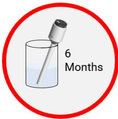
As soon as the running time of 6 months is reached, the hydrogen cartridge must be replaced immediately (see 4. Maintenance). Otherwise, a vacuum will form in the electrode and liquid can be soaked.
