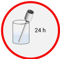
Place HydroFlex for 24 hours in distilled water. At least half of the shaft should be surrounded by water.
