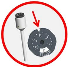
After 24 hours adjust the runtime to 6 months. For correct use do not change this. The hydrogen electrode is ready for your measurements.
