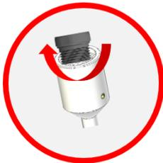
Screw the cartridge into the head of the electrode.
