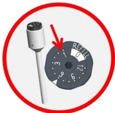
On top of the electrode head turn the runtime clockwise to position 1 with the operating runtime key or a 3 mm hexagon key. That is corresponding to one month.
